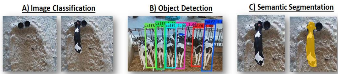
Figure 4. Image tasks using deep learning algorithms. Image Classification (Image A): classify if there is a calf in the image or not; Object detection (Image B): detect individual calves in the image; Semantic Segmentation (Image C): segmenting the calf body by detecting the pixels related to the target class (calf body).
